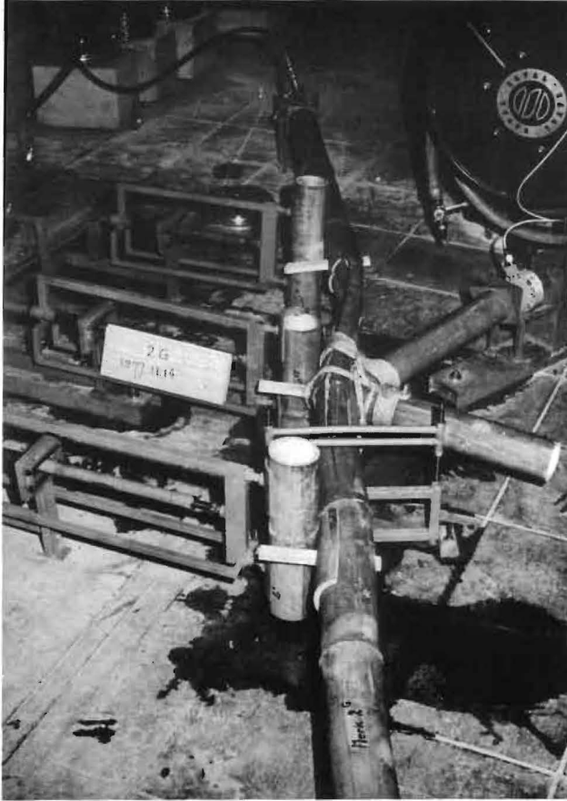
Picture 5.6.5. Joint 1.3., specimen G, after failure.
